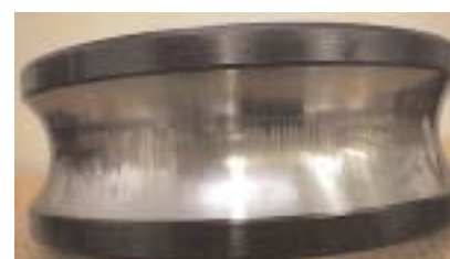
Fluting on failed bearing
