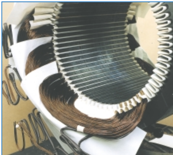
Figure 13: Partially wound stator core with random winding
